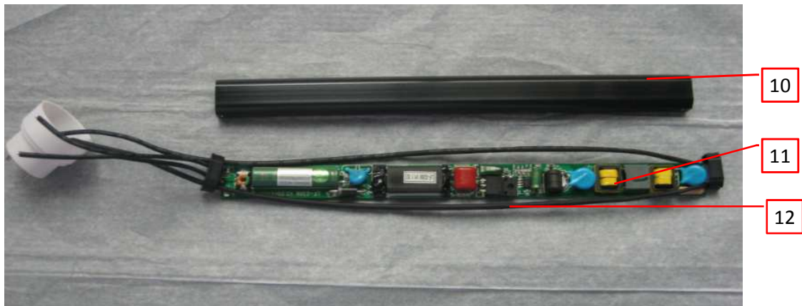
Photo 4 - LED driver view of model OH-GL-029
