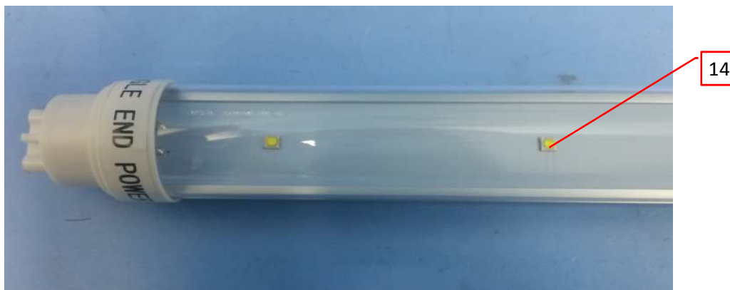
Photo 6 - LED PCB view of model OH-GL-022, OH-GL-021
